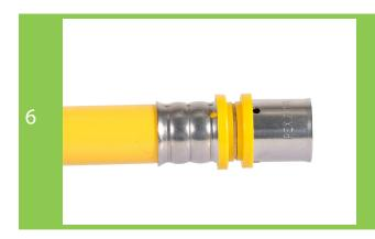
Stainless ring will have three visible lines it it has been crimped correctly.
