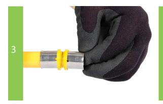
Push fitting into pipe until pipe is visible on the three viewing ports on the stainless steel crimp ring.
