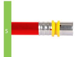
Stainless ring will have three visible lines if it has been crimped correctly.
