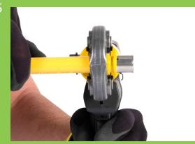
Proceed to crimp the fitting until jaws of tool are completely closed.
