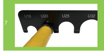
Once crimp is complete, test with gauge. Gauge will slide over stainless ring if it has been completed correctly.
