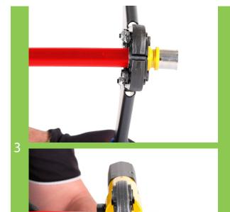
Using the STESSO crimping tool which has a 'U' profile jaw. Place tool over stainless steel crimp ring ensuring jaws are centred.
