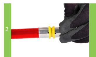
Push fitting into pipe until pipe is visible on the three viewing ports on the stainless steel crimp ring.
