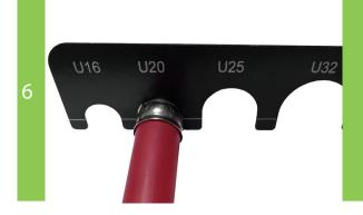
Once crimp is complete, test with gauge. Gauge will slide over stainless ring if it has been completed correctly.
