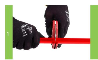
With a set of pipe cutters /shears cut the pipe at 90° ensuring the pipe is square on the end.
