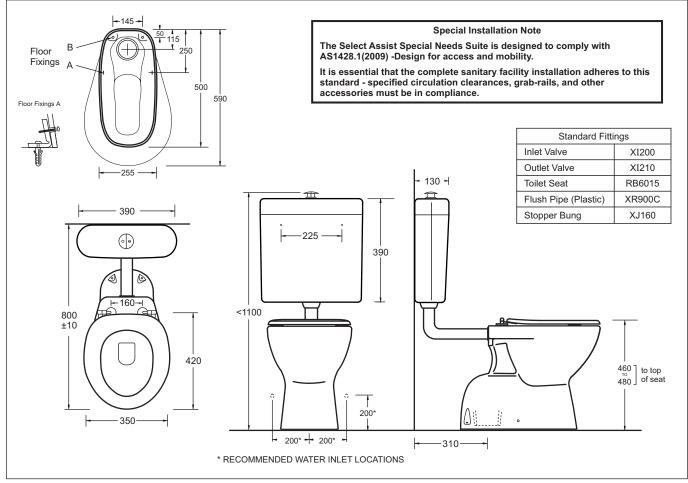
All dimensions are in millimetres and are subject to normal manufacturing variation of +/- 3mm on all surfaces. As product development is ongoing BPA reserves the right to vary specifications without notice. Bathroom Products Australia PILABN 87 079 297 617
