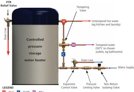
Caution: Water escaping from the drain line may be hot and could cause scalding. This valve is a Safety Valve. Excessive discharge from the drain line or operation of the small auxiliary relief valve opposite the drain can mean a malfunction within the system. Switch off the energy source and call a plumber or service person.
