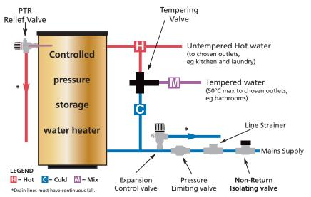
**TYPICAL CONTROLLED PRESSURE HOT WATER SYSTEM INSTALLATION**
