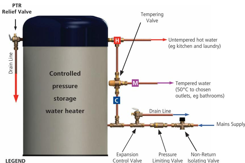
Caution: Water escaping from the drain line may be hot and could cause scalding. This valve is a Safety Valve. Excessive discharge from the drain line or operation of the small auxiliary relief valve opposite the drain can mean a malfunction within the system. Switch off the energy source and call a plumber or service person.
