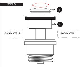
Screw Plug Mechanism (a) into Waste (c) and check for leaks.
