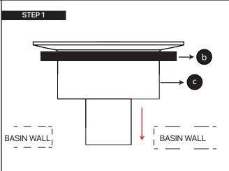
Thread Foam Washer (b) onto Waste (c) body and insert into basin hole.
