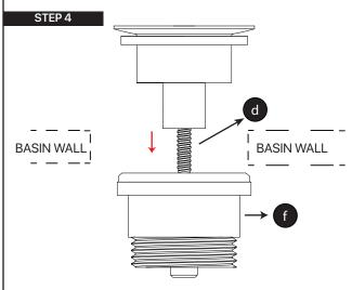
Locate Housing (f) underneath basin hole and screw in Housing Screw (d) from top and tighten firmly.
