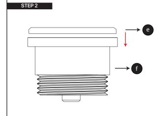
Insert Silicone Washer (e) into top of Housing (f).
