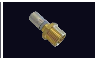
BRASS MALE ADAPTOR M12B - 1/2" BSP x 12mm
