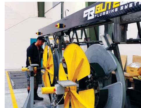
Manufacturing coils on the Buteline Pipewinder Buteline pipe lengths
