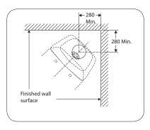
**45° Corner Set up** with arm support system
