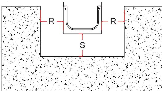
Table 1. Recommended thickness for subgrade and concrete abutments according to load classes
