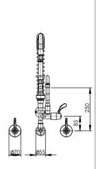
Spray trigger position dimensions are approximate and represent a brand new unit, spring will sag with use over time
