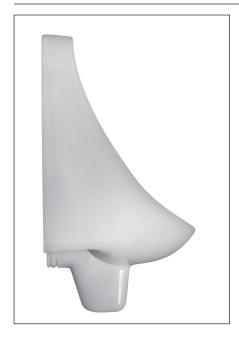
A general application wall hung urinal with integral trap. An adjustable spreader is suitable for installations with increased cistern head height. The spreader channels water to the front and back areas providing a wash down of the bowl on each flush.
