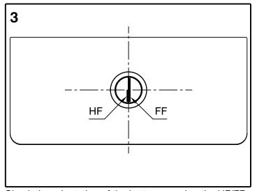
Check the orientation of the button ensuring the HF/FF markings on button are perpendicular to the back wall.
