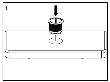
Fit the Button assembly into the cistern lid while keeping the half flush line to the left, as shown.
