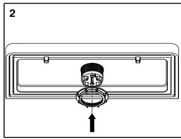
Screw the nut on the button assembly from underneath the lid.
