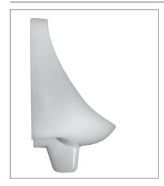
A general application wall hung urinal with integral trap. An adjustable spreader is suitable for installations with increased cistern head height. The spreader channels water to the front and back areas providing a wash down of the bowl on each flush. Available with back inlet and with a stainless steel grate as standard. Concealed cistern and plumbing fittings provide space saving, ease of cleaning and performance matched components to maximise low volume flushing efficiency.
