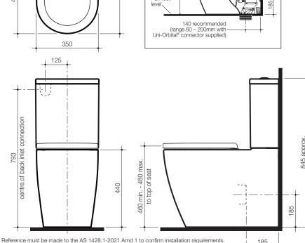
Adjust bedding height to ensure top of seat to finished floor height is in 460mm to 480mm range.
