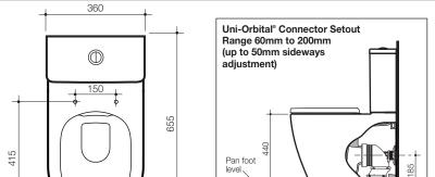
Urbane II Cleanflush™ **Wall Faced Close Coupled Toilet Suite with Chrome** Cistern Button and Seat with Stainless Steel Seat Caps 4.5/3 litre Back Entry Internal Overflow with inVogue
