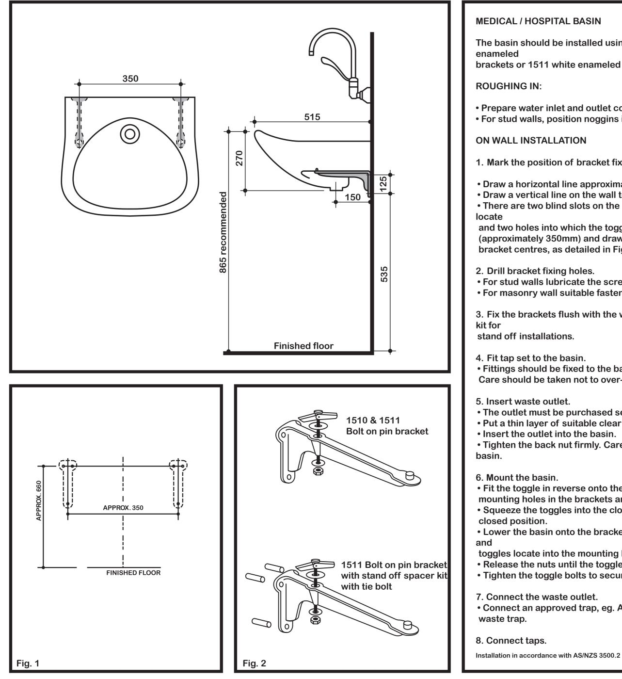
The basin should be installed using either a pair of 1510 uncoated alloy brackets, 1511 white
