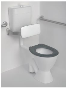
A pedestal type 4.5/3 litre dual flush Care 100 toilet suite installation designed to provide a raised seat height of between 460-480mm for accessible applications &. The versatility of the Care 100 suite makes it ideal for use by both the ambulant people with disabilities and wheel-chair users including wheeled commode chairs.
