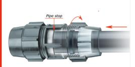
Twist the pipe into the fitting through the nut and split ring until it meets the first resistance pushing against the captive O-Ring.
