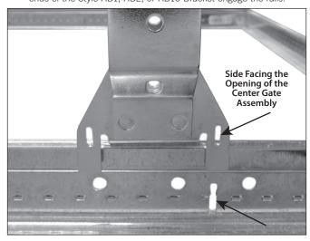
1a. For center-of-tile installations, align the end bracket with the center-of-tile slot of the T-bar rail (with the side facing the opening of the center gate assembly), as shown above.
