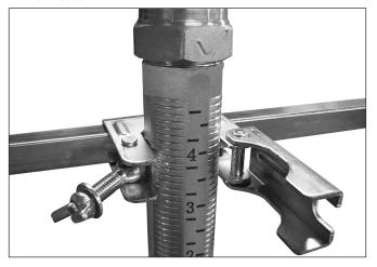
2. FOR STYLES AB1 AND AB10 BRACKETS ONLY: Move the center gate assembly of the Style AB1/AB10 Bracket to the desired location. Loosen the wing nut to open the center gate assembly, then slide the sprinkler reducing nipple into the center gate assembly. NOTE: The pivot screw of the center gate assembly is staked to resist removal of the wing nut.
