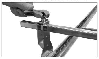
FOR STYLES AB1 AND AB2 BRACKETS ONLY: For adjustment purposes, the wing screw on top of the end bracket assembly can be loosened to allow the end bracket to slide on the square bar. Tighten the wing screw on top of the end bracket assembly to a torque of 36 inch-lbs/4 N•m (approximately ½ to ¾ of a turn past hand-tight) to secure the end bracket to the square bar.
