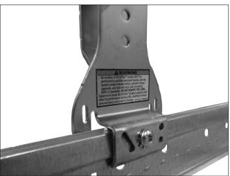
1b. Apply light downward pressure, as shown above, to maintain the position of the end bracket flat against the T-bar rail. To secure the end brackets to the T-bar rails, tighten the pre-installed sheet metal screws using a T25 drive bit. Penetrate through the T-bar rail until the end bracket is seated fully against the T-bar rail, as shown above. DO NOT over-tighten the screws. Over-tightening will cause the screw to strip, resulting in an unsecured bracket connection.
