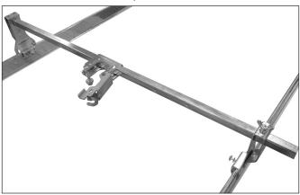
Attach the end brackets of the Style AB1, AB2, or AB10 Bracket to the T-bar rails of an ASTM C635 ceiling suspension system installed in accordance with ASTM C636 standards. Verify that the ends of the Style AB1, AB2, or AB10 Bracket engage the rails.
