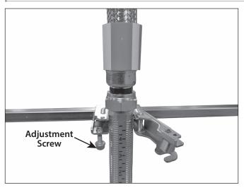
2a. FOR STYLE AB2 BRACKETS ONLY: Move the center gate assembly of the Style AB2 Bracket to the desired location. Using a T25 drive bit, loosen the adjustment screw, then push open the center gate assembly. Slide the sprinkler reducing nipple into the center gate assembly. NOTE: The adjustment screw of the center gate assembly is staked to resist removal.
