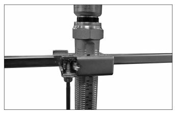
2c. FOR STYLE AB2 BRACKETS ONLY: Close the gate around the sprinkler reducing nipple. The gate will snap together tightly around the sprinkler reducing nipple. Using a T25 drive bit, tighten the adjustment screw to a torque of 75 inch-lbs/8.5 N ⋅ m (until adjustment screw makes metal-to-metal contact with bottom of gate). NOTE: The sprinkler reducing nipple can be adjusted after the drywall is installed by using the adjustment screw on the center gate assembly.
