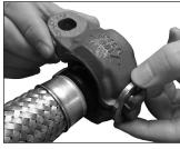
Install the linkage onto the housings, as shown to the left
