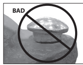
OVAL NECK OF BOLT NOT SEATED PROPERLY
