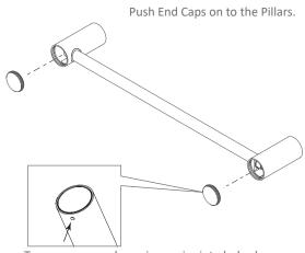
To remove cap, place pin or wire into hole shown and push firmly.
