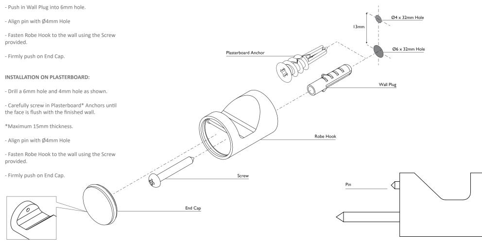
To remove cap, place pin or wire into hole shown and push firmly
