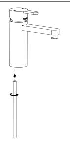
3 Screw the Red Marked Hose into the hole marked 'H' and the Blue Marked Hose into the hole marked 'C'.
