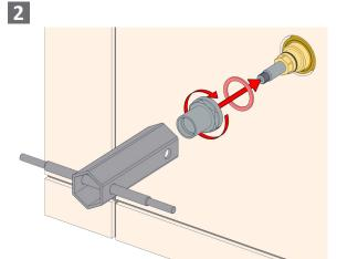
Fit Fibre Washer around the Cartridge, then firmly fasten the Bonnet onto the Cartridge using a Tube Spanner.
