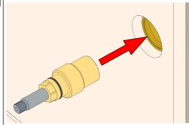
Firmly screw Cartridge into the Breach.
