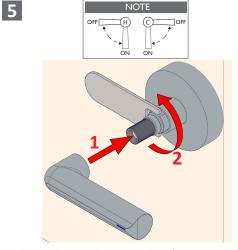
Push Handle onto the spline, then fasten Locking Nut to Handle, rotating counter clockwise using spanner.
