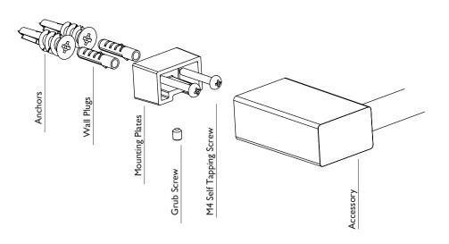
Place fixing plates where accessory is to be mounted. Mark center position of slotted holes.
