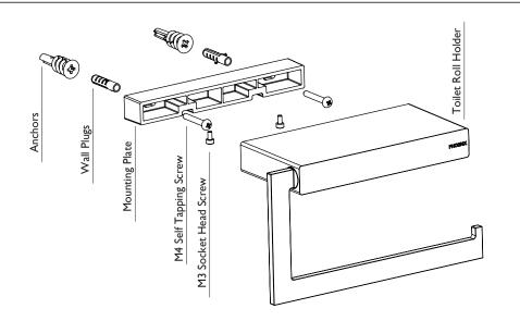
Place fixing plate where Toilet Roll Holder is to be mounted. Mark center position of slotted holes.
