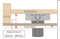
Adjustment range from Nogging Face to the Tile Face is 50mm to 68mm as shown.
