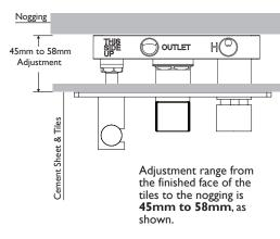
1 Screw the mixer breach to position. Ensure that the mixer breach is level.
