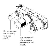
Connect hot and cold water supply, as shown.
