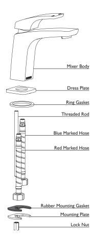
Cut a mounting hole 35mm in diameter. There must be a minimum 12mm width of flat around the hole.
