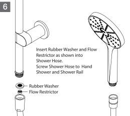
Test and check for leaks
