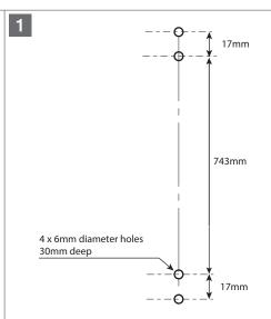
Drill into Wall Cladding 4 x 6mm diameter holes as shown on diagram
