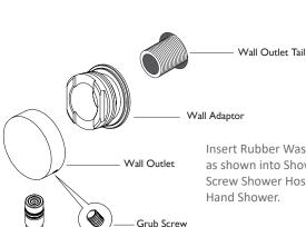
Insert Rubber Washer and Flow Restrictor as shown into Shower Hose Cone.
