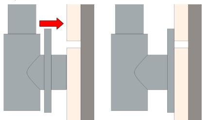
Screw on Overhead Shower Rose. WARNING! DO NOT REMOVE FLOW CONTROLLER. TEST AND CHECK FOR LEAKS.
