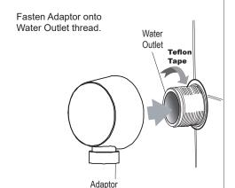
Ensure Rubber Washers and Check Valve are in places.
