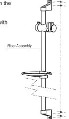
Drill mounting holes with 6mm drill bit.
