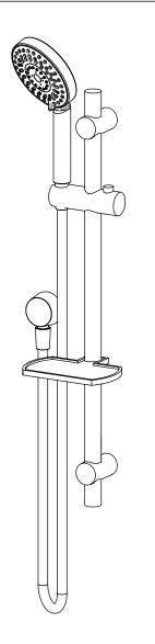
a) Measure and mark desired mounting positions. b) Drill mounting holes with 6mm drill bit.
