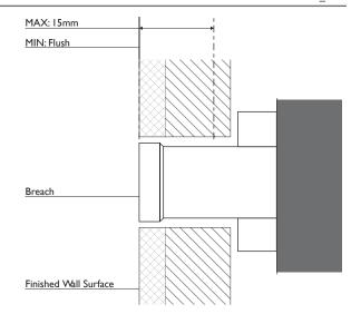
Firmly screw Spindle into the Breach.
