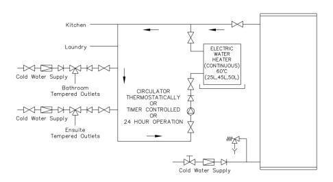
NOTE: A PLV IS REQUIRED TO BE INSTALLED ON THE COLD SUPPLY LINE
