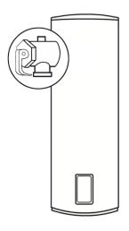
The expansion control valve will discharge the quantity of water from its drain line during the heating period instead of the temperature pressure relief valve as it has a lower pressure rating.
