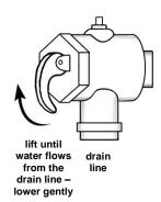
⚠ DANGER: Failure to operate the easing lever on the relief valve once every six (6) months may result in the water heater cylinder failing, or under certain circumstances, exploding.
