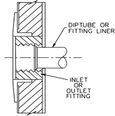
**LEFT AND RIGHT HAND SIDE WATER CONNECTIONS**
