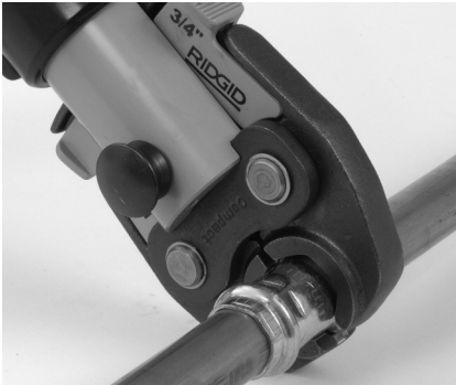
Figure 7 – Placing Scissor-Style Jaws Around Fitting
