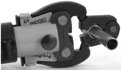
Figure 10 – Attaching Actuator to Press Ring
