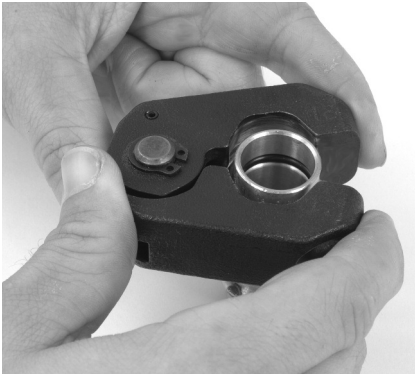
Figure 9 – Installing Press Ring onto Fitting
