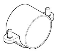
5. Make sure seal is correctly located in top half, with curved lip sealing on pipe.
