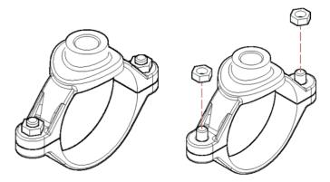
3. Hold bottom half underneath pipe. Ensure pipe area is clean, smooth and free from damage or defects.
