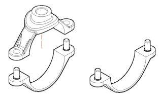
4. Place top half of Tapping Band over pipe. Locate bolt holes in top half into bolts in bottom half.
