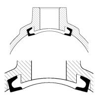
2. Remove top half and seal. Bolts are retained in bottom half by locating seals.
