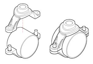
6. Tighten nuts evenly, maximum tightening torque 10-15nm. Take care not to damage or distort pipe.
