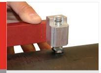
2. Adjust the scraper arm so that the indicator pin is flush with the upper end of the scraper blade holder.
