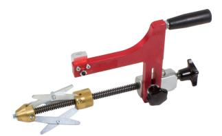
The Plasson Pipe End Peeler is the perfect tool for peeling pipes from DN63 – DN400. The engineered blade removes a consistent peel of oxidized pipe layer which is essential to a successful electrofusion weld.
