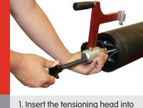
the pipe end and expand with the cross handle until it grips onto the pipe wall.
