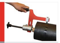
3. Rotate the scraper arm clockwise to remove a uniform layer of oxidized pipe.
