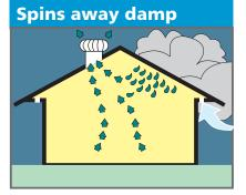
Under eave vents aid roof space air circulation. Install two per Spinaway.
