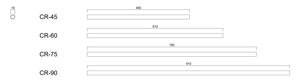
PLEASE NOTE: ONCE ROD IS PLACED INTO PILLAR ENDS, CTC'S OF COMPLETE RAILS ARE 450, 600, 750 AND 900mm
