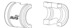
EXPANSION CONTROL GLOVE HALVES x 2 SETS (SECOND SET FOR PTR VALVE NOT SUPPLIED)
